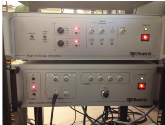
Figure 3.5: SPM control unit and High Voltage Amplifier
