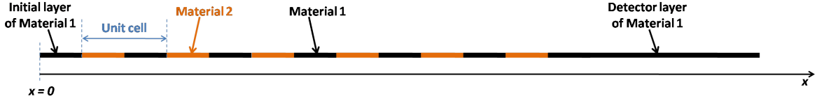
Figure 5.1: The super-lattice. The black segments represent the “Material 1”, the orange segments represent the “Material 2”. The used system of coordinate is indicated.
